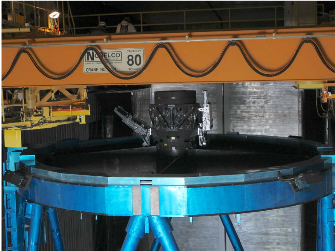
The center of this image shows the Prime Focus Camera (PFU), with the FEU (Filter Exchanger Unit) attached. (credit: NAOJ)
